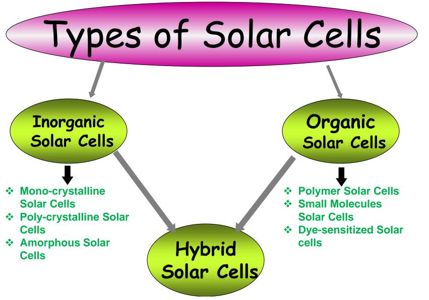
Brings together the advantages of both inorganic and organic solar cells. Inorganic particles (Ag, ZnO, FeS<sub>2</sub>, TiO<sub>2</sub>, etc.) are incorporated in organic materials. This may improve the efficiency and lifetime of solar cells.
