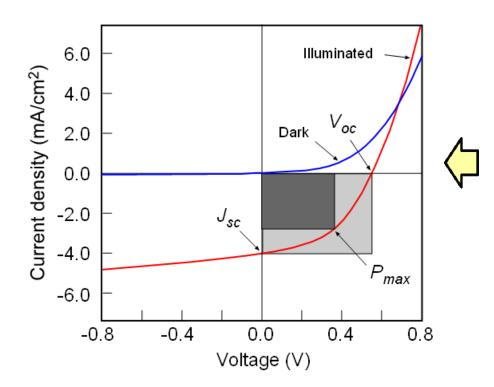
The typical *J-V* characteristics of an organic solar cell in dark and under light illumination
