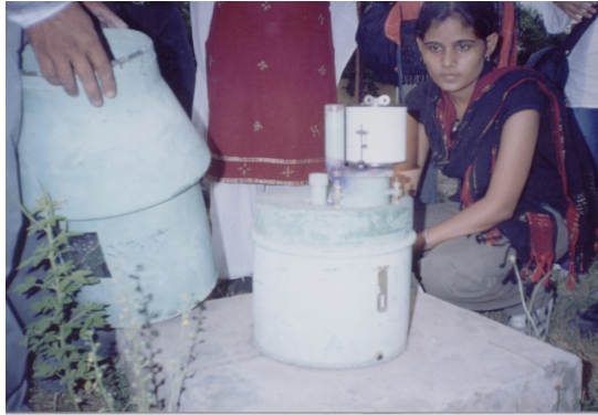
(a) Automatic Rainfall Recorder at Part-time Nowgaon Station, Chattarpur District
